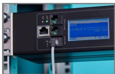
The PDU has a sensor port for connecting a digital temperature sensor, one dry switch contact or a combined sensor for temperature/humidity. The PDU registers which sensor is connected and automatically adapts the menu in the display to the sensor(s) that it has detected.
